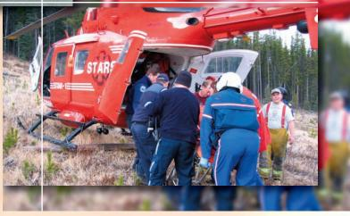
he BK117 is specifically designed for EMS operations and can be quickly loaded. The aircraft comes equipped with rear loading clam shell doors. The clam shells are opened while the aircraft remains running. The design of the main rotor system is such that it does not present a height hazard and the tail rotor is guarded by one of the two pilots.
